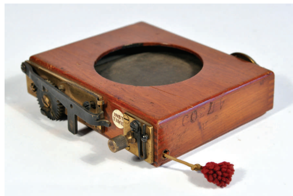
Thornton Pickards Time and Instantaneous shutter
